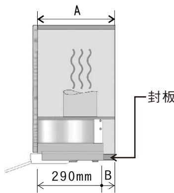
$$\text{※B} = \text{A} - 290\text{mm}$$
